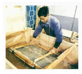
ABOVE (55) A modern demonstration of the traditional Chinese method of paper manufacture at the Ontario Science Centre. Here, the mesh screen mould is being lifted from the vat with its watery solution of disintegrated fibres. Although most paper in the modern world is made from wood pulp, the Chinese never used it, preferring the stronger fibres of linen and a variety of other plant materials, most of which would be too expensive for mass manufacture today.
